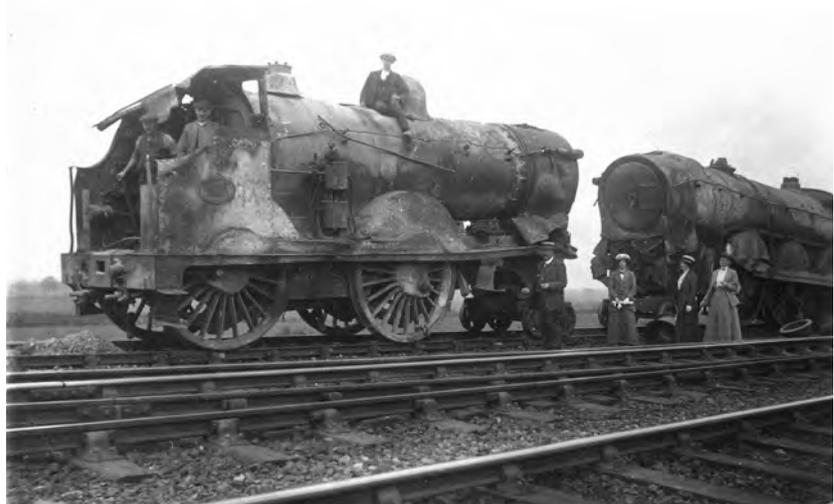
The two locomotives involved in the head-on collision: Caledonian Railway 4-4-0 No 121 and CR 4-6-0 No 907.
